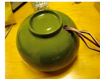
Drill a hole on the bottom of the bowl large enough to pull all four cables through.
