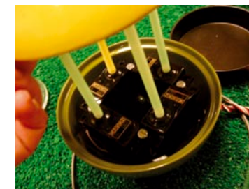
Drill four holes to put straws through bowl. Place four bendable straws on servo motor shaft.
